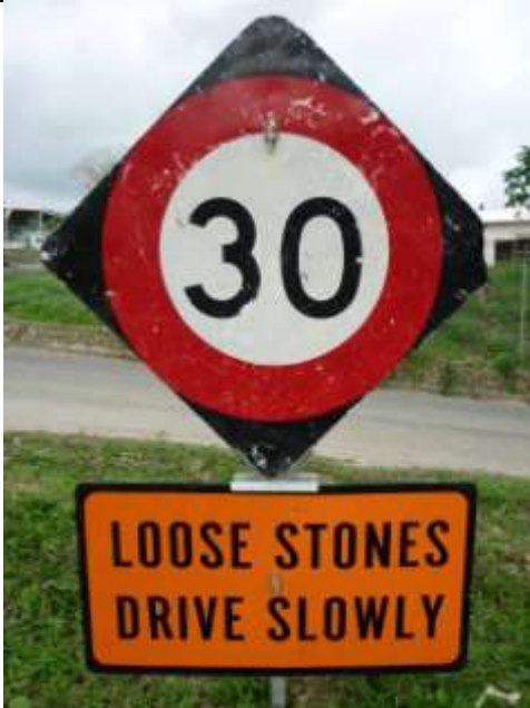
A sign that means what it says. This sign is placed on newly sealed sections and advises drivers that they should drive slowly because there are loose stones on the road. 30 km/hr is the speed limit.
