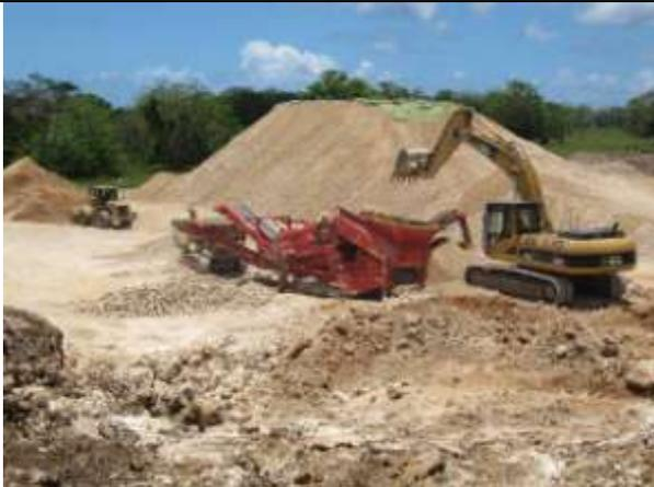
La Cressonniere Quarry in full production with 30 ton excavator and power screen in foreground and aggregate stockpiles in the background.
