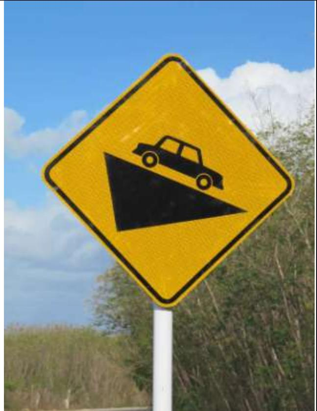
Steep Grade Sign – this is erected where vehicle speeds are likely to increase to an extent which would make a vehicle difficult to control. All trucks and loaded vehicles should change to a low gear before descending the hill.
