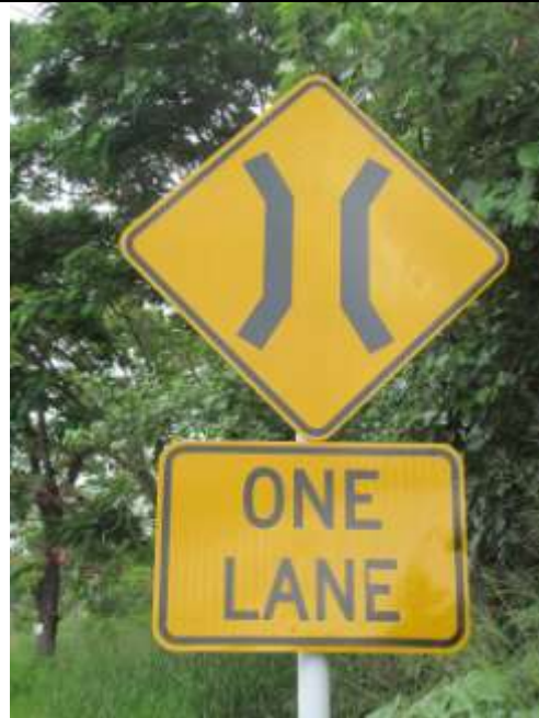
Narrow Road sign with One Lane supplementary plate. This means that the section of road ahead is only wide enough for one lane of traffic and that all vehicles need to proceed cautiously and be prepared to give way to oncoming traffic.
